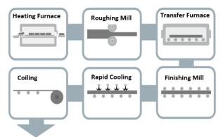
Hot Rolled Coil/Checkered Coil
