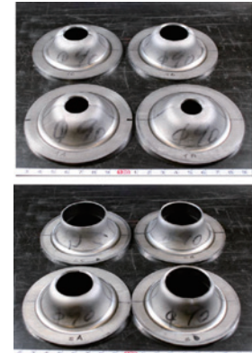
Photo2 Test pieces after hole expansion test (cylindrical type)
